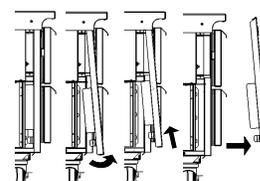
Vacuum or brush any dirt, lint or dust from the finned condenser coil, around the compressor and other cooling system parts as indicated. If significant dirt is clogging the condenser fins, use compressed air to blow this clear. When finished reverse the louver removal process as instructed above.
