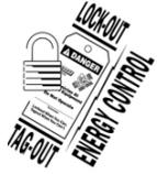
**⚠ WARNING** Certain procedures in this section require electrical test or measurements while power is applied to the machine. Exercise extreme caution at all times. If test points are not easily accessible, disconnect power and follow lockout / tagout procedures, attach test equipment and reapply power to test.
