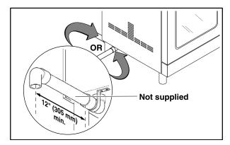
Figure 8: Drain Connection
