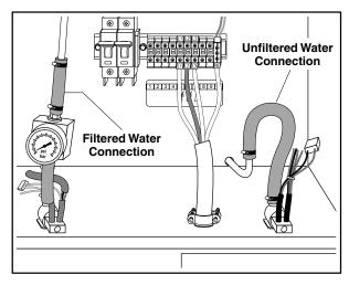
Figure 7: Water Supply Connections for CEM20U
