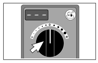
Figure 26: Internal Product Probe Temperature Selector Knob (if Installed)
