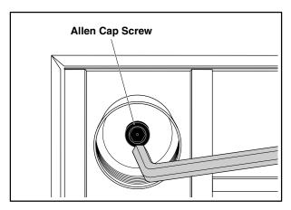
Figure 2: Allen Cap Screw Location
