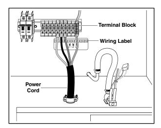
Figure 5: Power Supply Cable Connection
