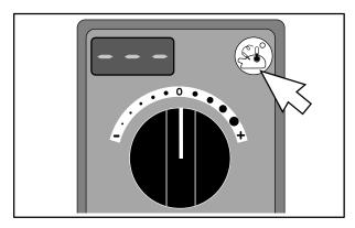
Figure 27: Internal Product Temperature Probe Button (if Installed)
