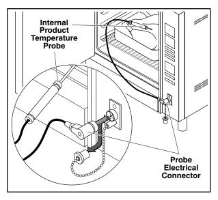
Figure 28: Cooking with the Internal Product Temperature Probe
