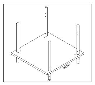
Figure 4: Assembled Combination Oven Stand
