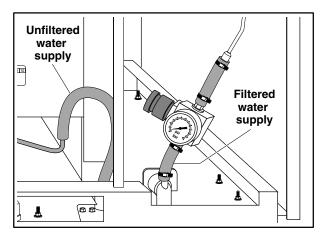
Figure 6: Water Supply Connection for CEM6U and CEM10U
