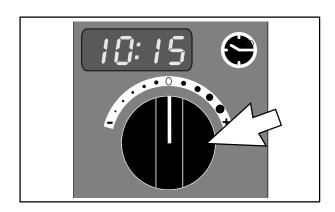
Figure 22: Oven Timer Adjustment Knob
