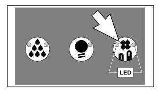
Figure 25: Fan Speed Selector
