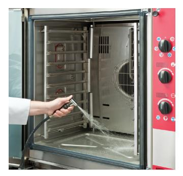
**STEP 5 - When finished steaming,** open the door and rinse the interior with the attached spray hose. Wipe down door gasket with clean towel.
