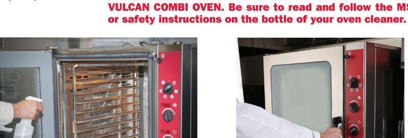
**STEP 3 –** Spray the oven interior with oven cleaner. Turn the nozzle to adjust the spray pattern.
