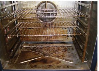
STEP 2 - Fill the spray bottle with a mild oven detergent. We recommend the following cleaners: Greasecutter Plus by Ecolab, EZ Clean by Cello, or Advance Oven Cleaner by Diversey-Lever. DO NOT USE ABRASIVE CLEANERS OR CHLORIDES ON YOUR **VULCAN COMBI OVEN. Be sure to read and follow the MSDS**
