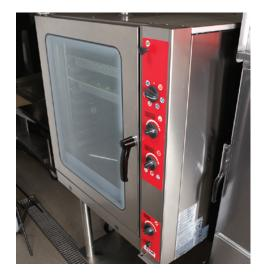
**STEP 1 -** Place the oven in cool down mode. Let the oven cool to below 140°F (60°C).
