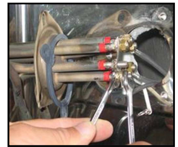
Element electrical connections seen from the rear of the oven
