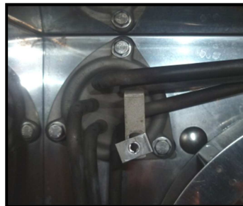
Element electrical connections seen from the rear of the oven
