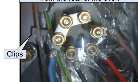
Element electrical connections seen from the rear of the oven
