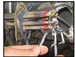
Element electrical connections seen from the rear of the oven
